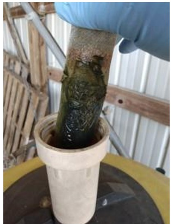
Figure 2. Check strainers regularly and clean or replace them as needed (Photo: Ric Bessin, UK).
